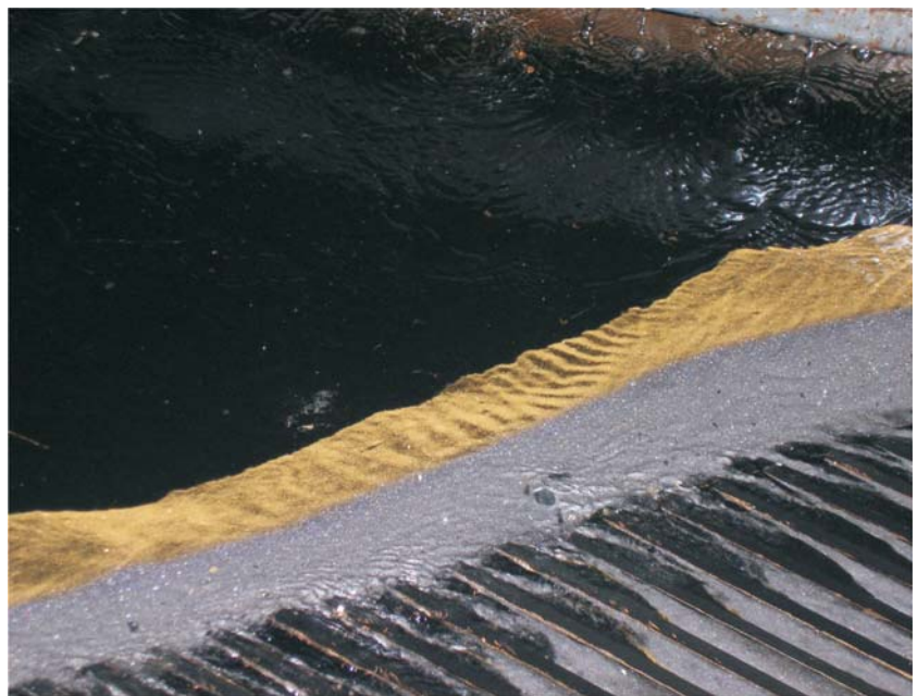
Final concentration on a shaking table
