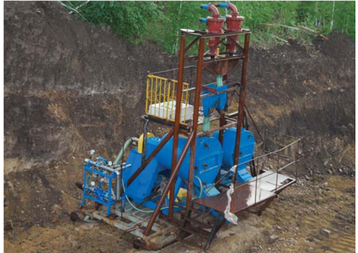
Twinned ITOMAK installation treating tailings, Zabaykalye
