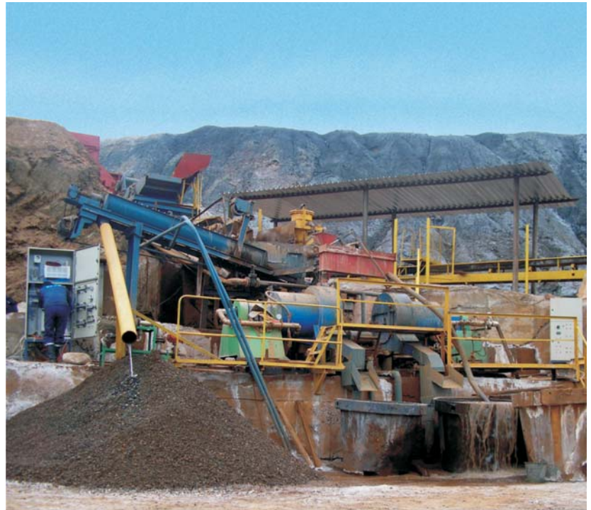
Automated ITOMAK unit for the fine gold recovery, Kyrgyzstan
