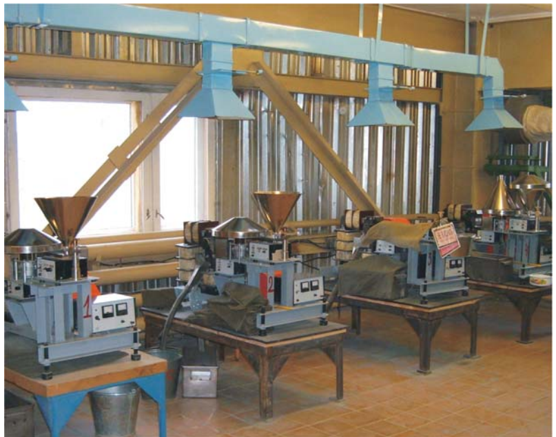
Line of magnetic separators at ALROSA recovery plant
